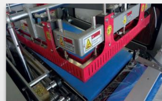
Product infeed conveyor /Film forming shoulder
