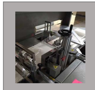
Side Sealing (upstream)
